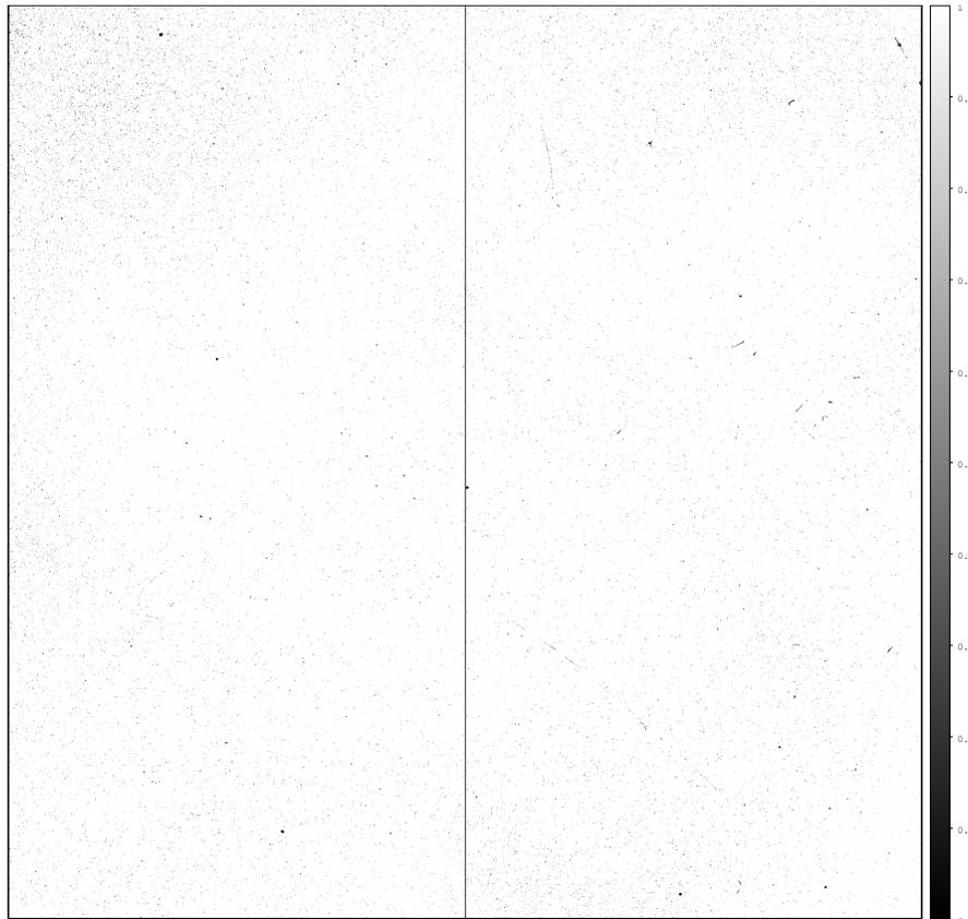
**Figure 23.** This figure shows the quantum efficiency operability map at K-band, where white is operable and dark is inoperable. The quantum efficiency limit for operability is  $> 70\%$ . The number of operable pixels is 99.3965 % or 4136484.
