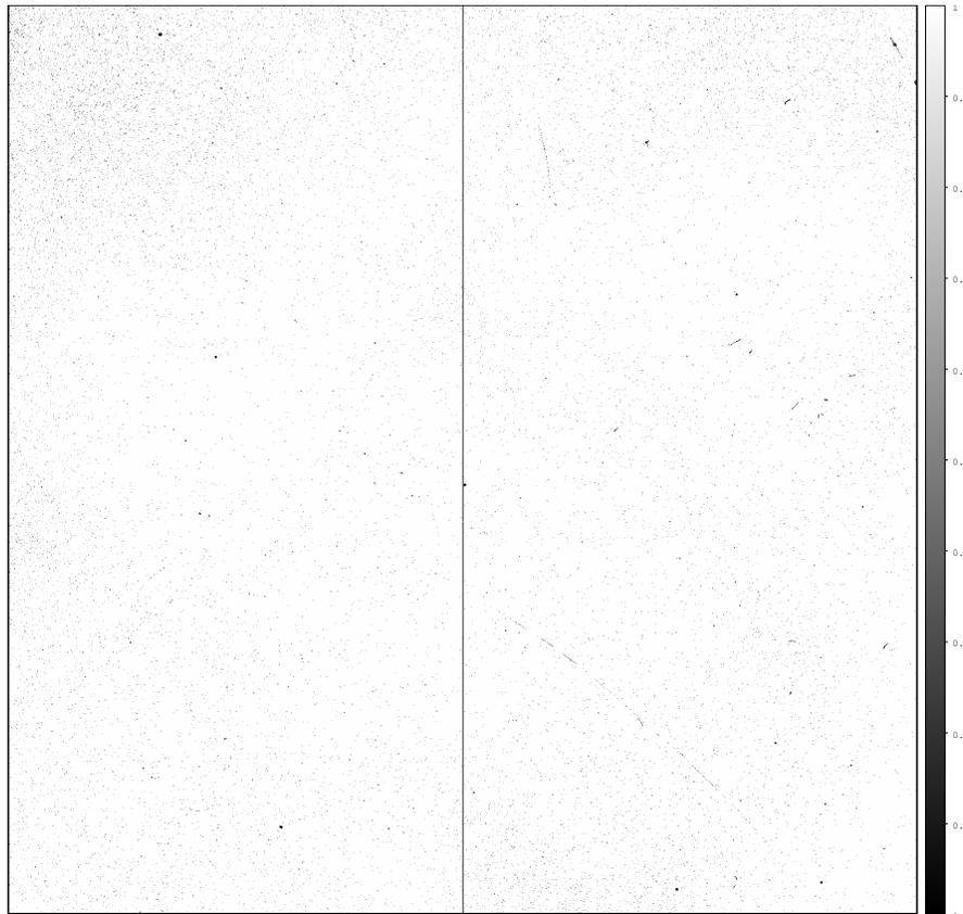
**Figure 21.** This figure shows the quantum efficiency operability map at J-band, where white is operable and dark is inoperable. The quantum efficiency limit for operability is  $> 70\%$ . The number of operable pixels is 99.3086 % or 4132828.
