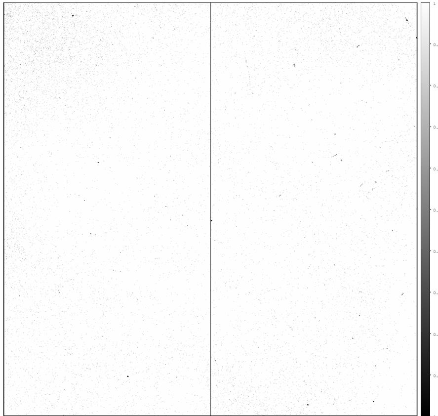
**Figure 22.** This figure shows the quantum efficiency operability map at H-band, where white is operable and dark is inoperable. The quantum efficiency limit for operability is  $> 70\%$ . The number of operable pixels is 99.5756 % or 4143939.
