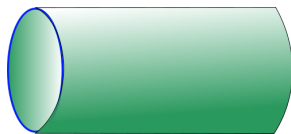
Figure 5: The rate that mass of the fluid is swept up \frac{dM}{dt} = \rho Av where A is the cross sectional area, \rho is the density of the fluid and v is the velocity. The rate of momentum change is \frac{dp}{dt} \sim \frac{dM}{dt}v = \rho Av^2 . The drag force scales with these physical quantities.
