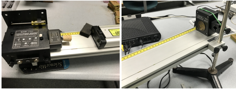
Figure 2: The lab setup. Left: The force center is held by a bumper holder. A cork is held onto the bumper with a piece of double sided tape or a glue dot. Right: the right the track is held up by the stand so that it is slightly inclined. The motion sensor is held with a rubber band. I found I could not incline the track by more than a few degrees without going over the force sensor limits when the cart collides with the force sensor.
