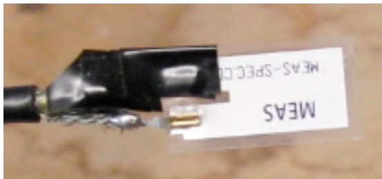
Figure 3. The lead connected to the inner wire in the coax cable has been covered with insulating electrical tape. However the other pin is bare. When you cover with copper conducting tape, the inner wire will not be shorted to the shield, and the tape will touch the shield. This way shield can cover the entire tab.
