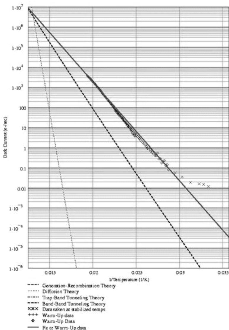
Fig. 11. Arrhenius plot of dark current as a function of inverse temperature for a  $2K \times 2K$  InSb array obtained by the University of Rochester.<sup>1</sup> The measured dark current follows a straight line on this semi-log plot down to 33 K and then flattens out to 0.01 electrons/second at 30 K. Data were obtained both during warming up and cooling down the detectors.
