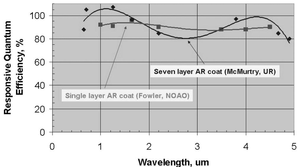
Fig. 7. QE of large-area InSb SCAs as a function of wavelength. The data obtained by Fowler at NOAO is from a  $1K \times 1K$  ALADDIN SCA with a single-layer, broad-band AR coating. The data from McMurty at the University of Rochester is from a  $2K \times 2K$  Phoenix SCA with a seven-layer AR coating designed to enhance visible response and maintain high QE in the infrared as well. The smooth curves are polynomial fits to each data set.
