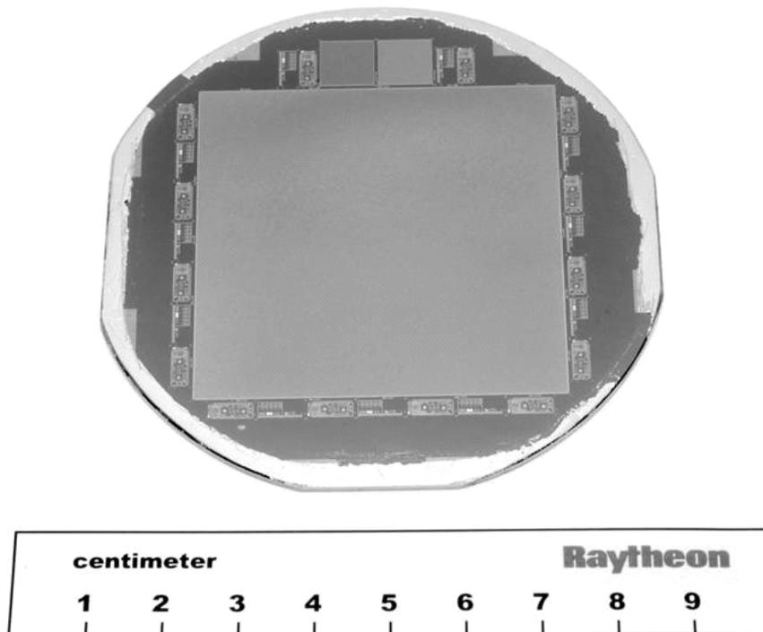
Fig. 2. Photograph of 82 mm diameter InSb wafer with a  $2048 \times 2048$  ( $2K \times 2K$ ) element array patterned on it. Each detector element is  $25 \mu\text{m}$  square. The small die surrounding the  $2K \times 2K$  array are various test structures.
