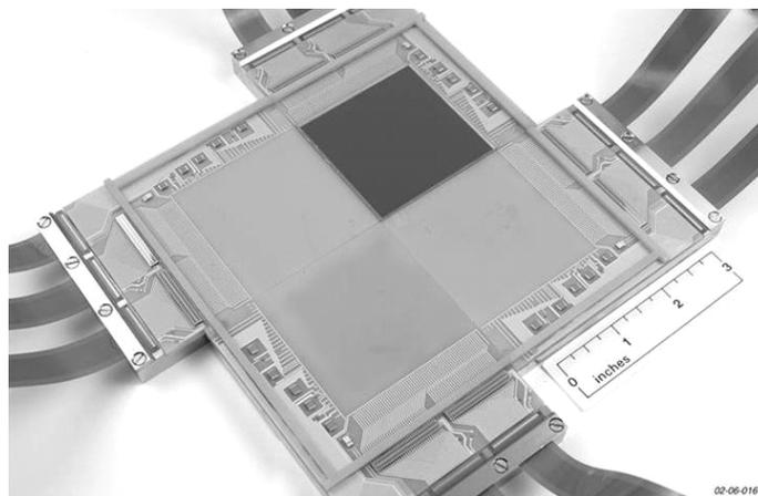
Fig. 5. A demonstration focal plane with four ORION modules. One module contains an InSb SCA while the others have bare readouts. This focal plane demonstrates the ability of the 2-sided buttable modules to create a  $4K \times 4K$  focal plane.
