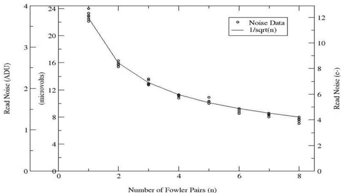
Fig. 9. Noise measured by University of Rochester on a Phoenix  $2K \times 2K$  InSb module using 100-second integrations.<sup>1</sup> The total noise—including readout, detector, and test set noise contributions—is shown as a function of the number of Fowler sample pairs. The noise follows the square root (number of Fowler pairs) relation predicted for uncorrelated white noise with 4 electrons noise measured for Fowler-8. The module temperature was 30 Kelvin.
