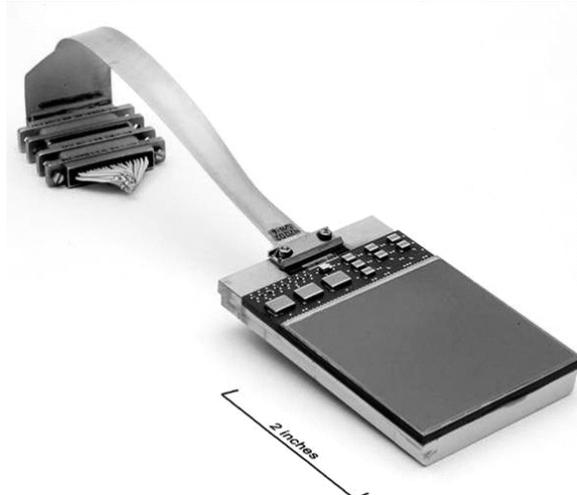
Fig. 8. The Phoenix  $2048 \times 2048$  ( $2K \times 2K$ ) InSb module. The InSb SCA occupies the majority of the module surface. A temperature sensor, current-source resistors, and noise-reduction capacitors are located on the upper-left of the module.
