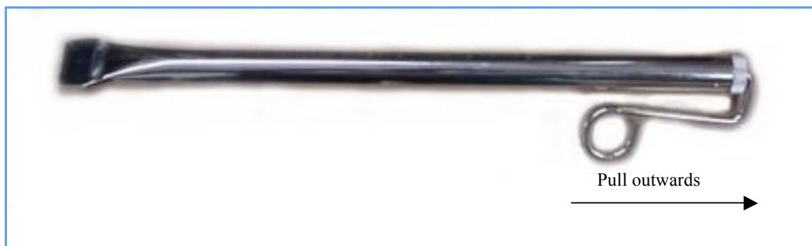
Figure 1. Above is an example of a metal sliding whistle. When pushed all the way in, I find that the distance between the end of the inner stopper inside the tube and the edge of the hole in the mouth piece is about 3.8 cm. As the stopper is pulled outwards this distance increases. When you blow into the whistle you get a high note if the stopper is nearly all the way in. As you pull out the stopper the note becomes lower and lower.
