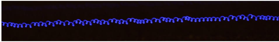
Fig. 5. A photographed trajectory illustrating period doubling and tripling. This is a trajectory of a somewhat more massive mechanism (1.7g) with a larger displacement ( A \sim 0.5 mm), a frequency of 240Hz and on cornmeal.
