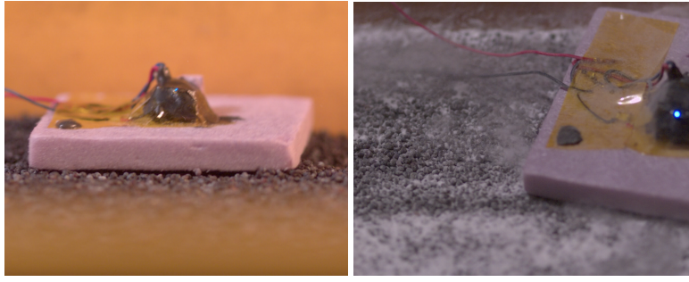
Fig. 6. Placeholder for two high speed videos. Both show the same mechanism traversing poppy seeds and filmed at 1000 frames per second. The poppy seed substrate has been covered with a layer of cornstarch in the second video. Videos are temporarily viewable here https://youtu.be/kLsG6e_-IqM .
